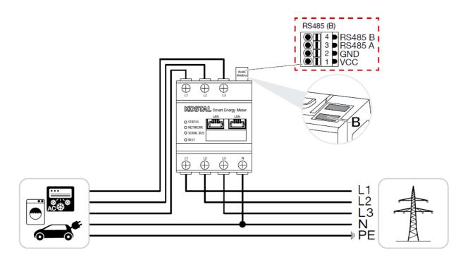
Settings in the KOSTAL Smart Energy Meter are not necessary as this is preconfigured on the RS485 B interface for the coolcept fleX /coolcept<sup>3</sup> fleX.
