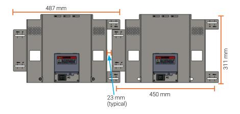
BWM-600MM-A allows 600 mm battery-to-battery spacing:
